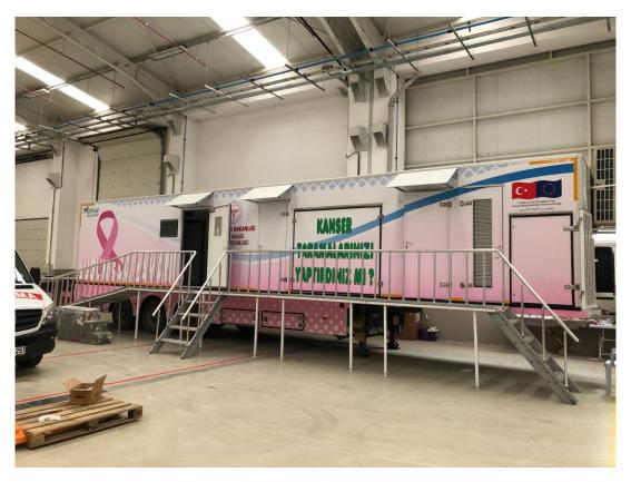
Mobile cancer screening tools are only used for cancer screening purposes. According to the usage needs, the trailer contains energy, device, device connections and is produced with lead plates insulated in order to protect from radiation in TAEK standards. In addition, the trailer is equipped with the necessary equipment such as tables, chairs, waiting rooms and sinks in accordance with its relevant purpose.
